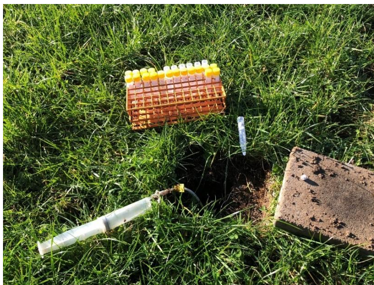
Figure 13 Collection of leachate samples from ceramic suction cups.
